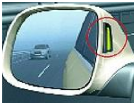
Figure 4: Signal warns driver if a car is in the blind spot (Smartmicro).
